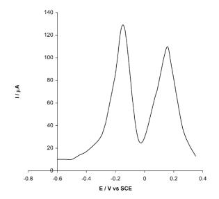
Fig. 2. Simultaneous determination of ascorbic acid and  $\alpha$ -tocopherol (200 µg cm<sup>-3</sup>:75 µg cm<sup>-3</sup>) in 0.1 M TX-100 + 40% (v/v) acetonitrile + water mixed solvent systems at a scan rate of 2 mV s<sup>-1</sup> and pulse height 100 mV.
