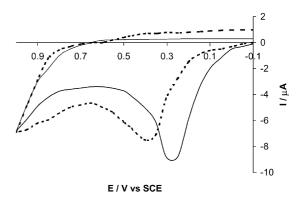
Fig. 1. Cyclic voltammograms for  $2.53 \times 10^{-4}$  M  $\alpha$ -tocopherol (—) in pure ethanol and (---) 0.1 M CPC + 50% (v/v) ethanol + water mixed solvent systems.
