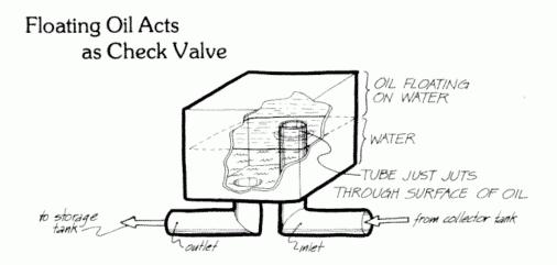
Functionally, the oil valve acts just like a check valve. It lets the hot water flow through in one direction but not in the reverse direction. Coupled with the thermosyphon circulation between the collector tank and the storage tank, the oil valve lets *heat* flow one way, but not the other. Thermosyphon circulation and the oil valve provide the same diode function that the controller and pump does in the active system.
