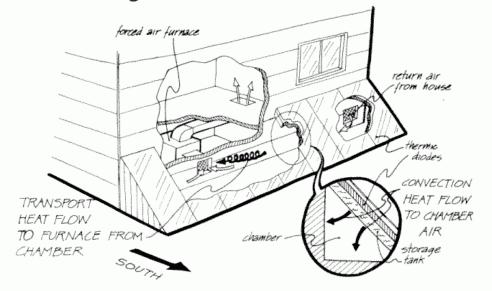
In either hot-water heating or house heating, this passive system separates storage from both the collector (reducing nighttime heat loss) and the living space (allowing heat to be delivered only when it's needed). It performs both the diode and the control functions.
