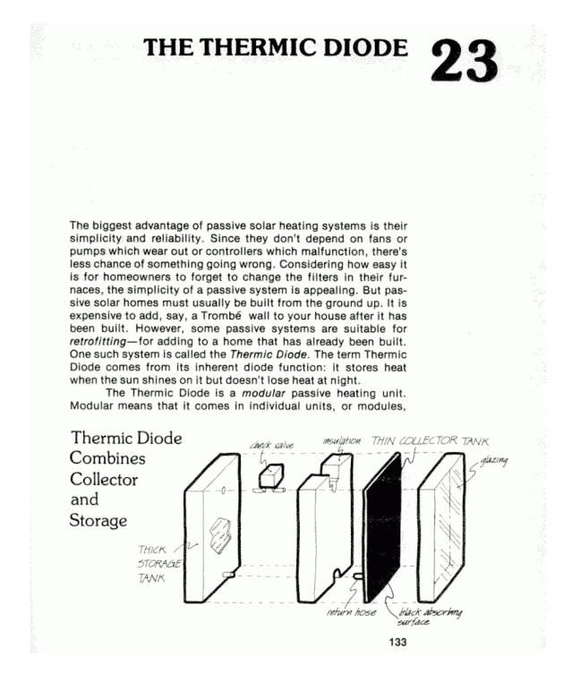
which can be mass-produced in a factory as the collectors of active solar heating systems are. But it is also passive; it has no fans or pumps and requires no electricity to operate. Each module contains a complete solar heating system: a solar collector, a controller, a heat storage unit, and even a heat exchanger. Yet the Thermic Diode is simple, rugged, and reliable. It doesn't even have any moving parts that could blind or corrode.
