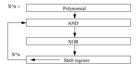
The idea is that, by using these numbers as binary constants, that define the XOR feedback around a shift register, the shift register will cycle though all the non-zero values, that can be represented in as many bits. The sequence generated is of a maximal length, ie 2^n-1 values.
