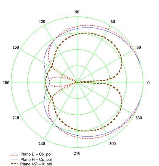
Fig. 5. Radiation diagram for the waveguide WR112 partially filled with dielectric layer
