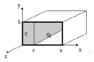
Fig. 1. Rectangular waveguide partially filled with dielectric.
