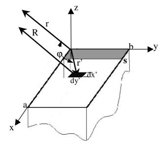
Fig. 2. Open-ended partially filled waveguide radiating in free space.
