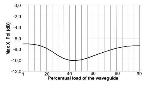
Fig. 4. Maximum cross-polarization as a function of the dielectric loading, s. Rectangular waveguide WR112 (a = 2.850 cm and b = 1.262 cm).  $\epsilon_r$  = 2.32.
