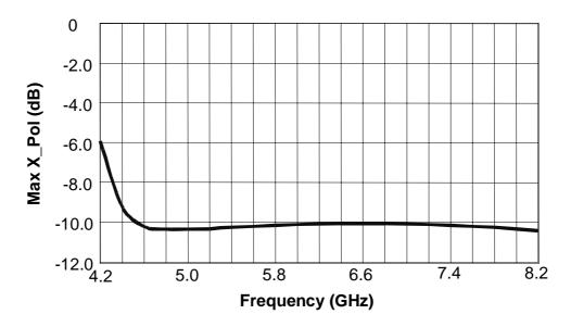
Fig. 6. Maximum cross-polar level as a function of frequency in the waveguide WR112, partially filled with dielectric,  $\varepsilon_r = 2.32$ . s = 0.45a. Radiation plane  $\phi$ =45°.
