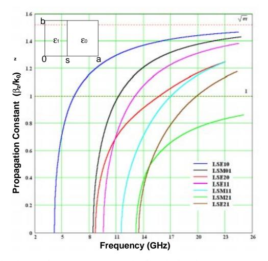
Fig. 3. Dispersion curves for the waveguide WR112 partially filled with dielectric layer with  $\varepsilon_r = 2.32$ . s = 0.45a.
