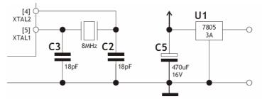
The system is supplied a 6 Volts DC current, we use a 7805 to stabile the voltage to 5 Volts DC. The microprocessor is running on an 8MHz crystal so the pulse measurement is in microseconds (us).
