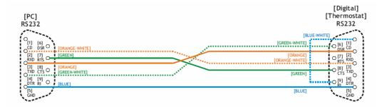
The communication cable for the connection between PC and Digital Thermostat is as in the picture above.
