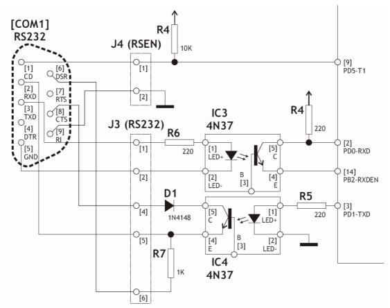
Now the AT90S2313 sends the 'Q' character on RESET that means every 2 seconds. The PC can send an 'R' Read or 'W' Write character command. On Read command the response is 'B' character and 40 bytes or 20 integers of the Parameters inside the AT90S2313. On Write command the response is 'S' character and now the AT90S2313 waits for the following information.
