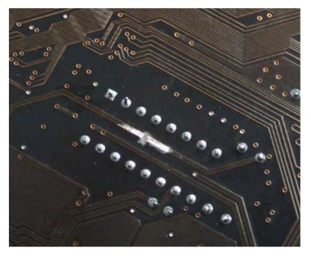
5) The trace on the back must be cleaned and broken as shown. Use a "Dremel" or other grinding tool to make a break in the trace and then clear off the soldermask to expose some copper on each side.
