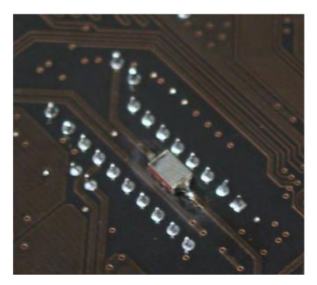
6) Then, install the ferrite bead across the broken trace. Make sure your solder does not touch any other pins, and make sure you have good contact.
