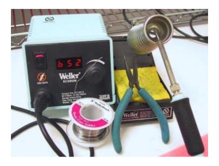
1) You will need some tools: Get a fine tip soldering iron, some fine rosin core solder and very fine needle nose pliers or tweezers. I also recommend some stong reading glasses to see the tiny parts better.
