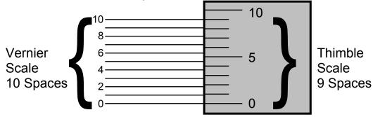
The difference between a space on the vernier scale and a space on the thimble space is 0.0001 inches. When reading a vernier micrometer, the first three steps are the same as for a regular micrometer. We will then add a fourth step:
