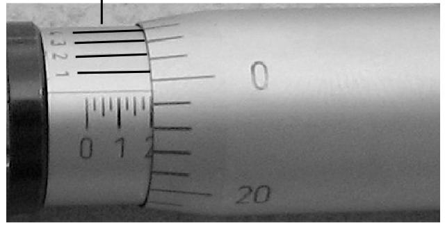
The total distance of the ten vernier scale spaces is equal to the total distance of nine scale spaces of the thimble scale:
