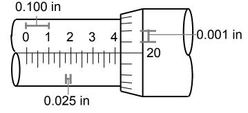
There are four steps we follow when reading an inch-system micrometer. **Reading an Inch-System Micrometer:**
