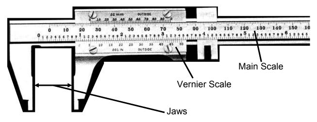
Much like the inch-system micrometer, each inch of the main scale is divided into forty equal parts meaning that the smallest division on this
