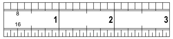
On the top, each inch is split into 8 equal parts. Thus, the 8 indicates the length between two successive marks is one-eighth of an inch. On the bottom, each inch is split into 16 equal parts. Thus, the 16 indicates the length between two successive marks is one-sixteenth of an inch. Let's try reading some measurements:
