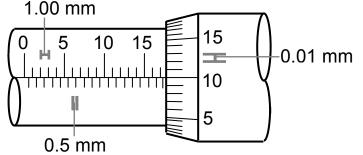
There are four steps we follow when reading a mm-system micrometer.
