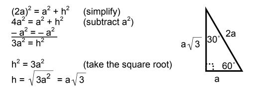
This means that the ratio of sides for a 30°-60°-90° is a:  $a\sqrt{3}$ : 2a.
