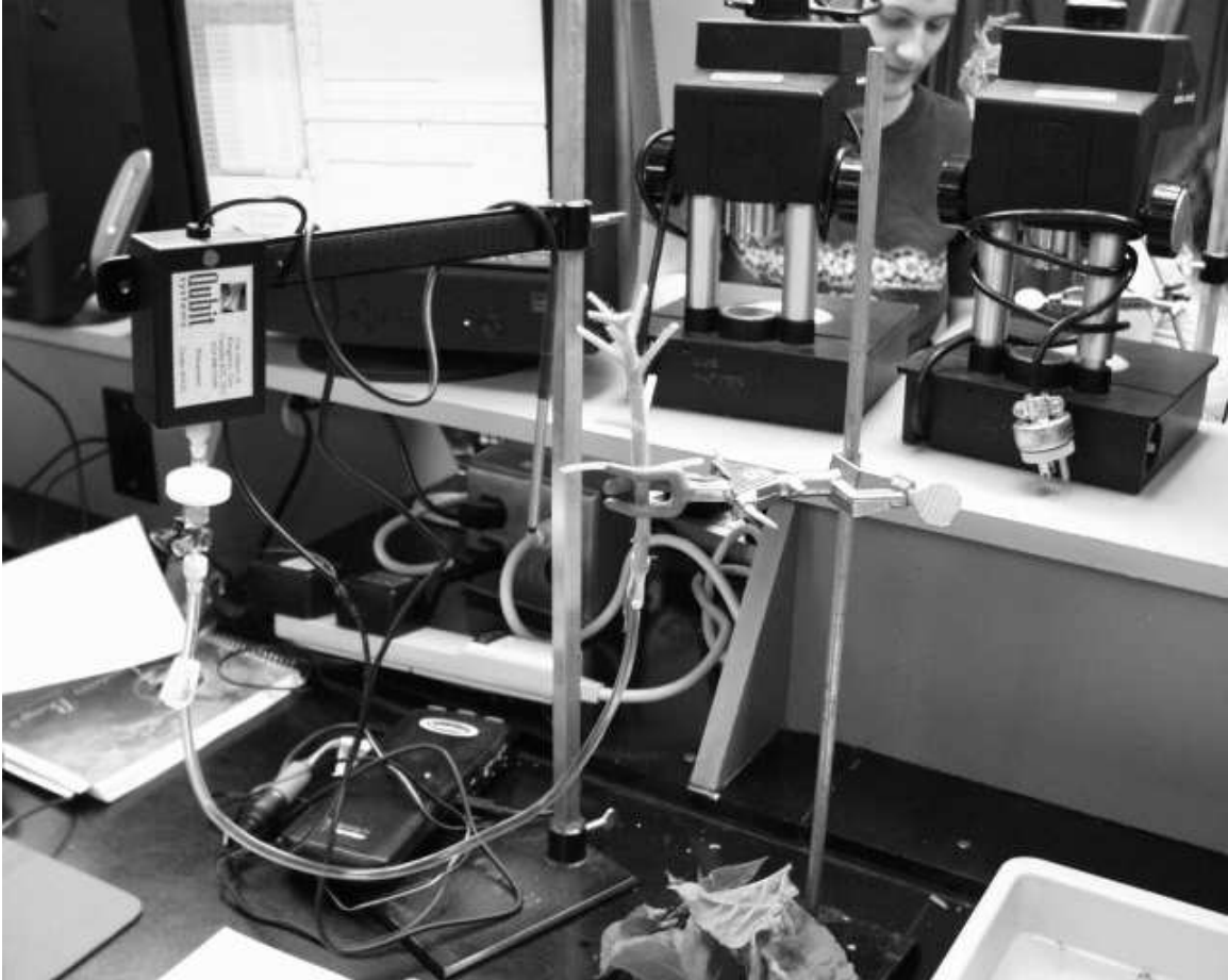
Figure 1: Example of Qubit Systems Electronic pressure sensor, water-filled connecting tube, and electronic temperature sensor
