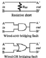
Fig. 13. Wired-And and Wired-OR Fault Models
