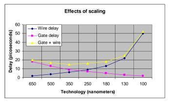
Fig. 7. Effects on scaling on circuit delays
