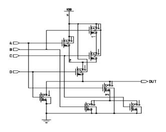
Fig. 3. Complex gate (D + A (B + C))'. Lines 1, 2, and 3 denote lines that were shorted in different combinations with the inputs.
