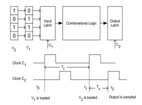
Fig. 6. Hardware model with clock timings
