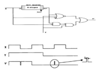
Fig. 10. Logical level model for crosstalk pulse fault using shift registers as transition detector
