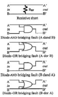
Fig. 17. Diode-And and Diode-Or Bridging Fault Models
