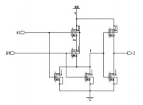
Fig. 1. CMOS OR gate. Lines 1 and 2 denote lines that were shorted in different combinations with the inputs.
