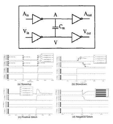
Fig. 9. Inverter-Capacitor model for Crosstalk and 4 transient effects modeled by it
