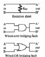
Fig. 13. Wired-And and Wired-OR Fault Models
