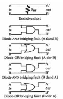
Fig. 17. Diode-And and Diode-Or Bridging Fault Models
