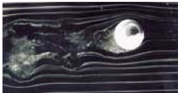
Figure 4: Flow Diagrams for a Non-Rotating Sphere
