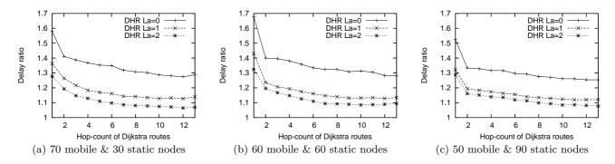
Figure 12: The ratio of the delay of the DHR (with different  $L_a$ s) routes to that of the Dijkstra routes in networks of different numbers of mobile nodes and static nodes.
