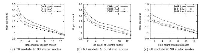
Figure 10: The ratio of the hop-count of the DHR (with different  $L_a$ s) routes to that of the Dijkstra routes in networks of different numbers of mobile nodes and static nodes.
