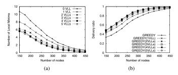
Fig. 1. Effectiveness of the virtual long links in reducing the number of local minima. 2 VLLs means 2 virtual long links per node (a) & Delivery ratio in pure greedy routing protocol (b).
