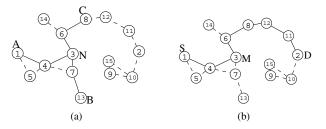
Fig. 2. The virtual long links of node N (a) & Pure greedy routing with virtual long links (b).
