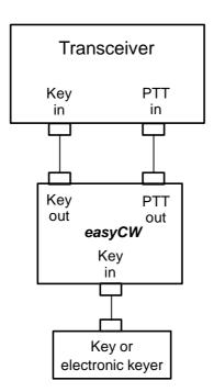
Plase note that the internal transceiver semi break-in shall be deactivated (i.e. VOX set to OFF), or even left on but with the delay set to minimum.
