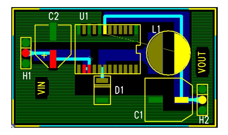
The reason I made this board is too be able to use one battery to drive my motors on a small robot. The input power from the battery could be anywhere between +7 volts D.C., and +24 volts D.C. The output from this board is a nice stable +5 volt D.C. suitable for driving microprossecrors, and logic circuits, it is capable of providing up to 1 amp of power. Which is more then enough to run most Microprocessor boards. Another nice feature is
