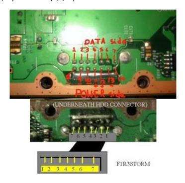
Be sure to solder the wires to the correct points as labeled in both pictures, and do not bridge any solder points, or you might brick your Xbox 360.
