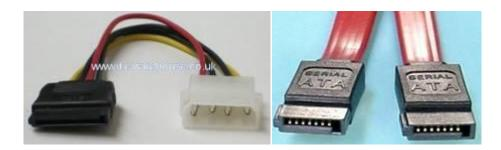
The top picture is a Molex>SATA power adaptor. The bottom picture shows a SATA cable. You can use this Molex>SATA to power your Xbox 360 hard drive, and the SATA cable to connect the hard drive, of course after disassembling the hard drive casing. This is a picture of my HDD connected to my PC using a SATA cable and a MOLEX>SATA cable.
