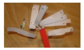
After that cut down the yellow and black wires which are 12volts. The red and black are 5 volts and these are what the HDD will use. (See picture below)
