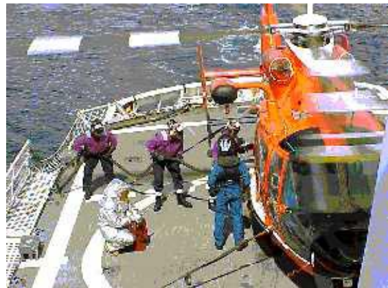
USCGC RELIANCE engineers refueling an HH65 Dolphin Helicopter. The 3 man refuel team pump away and DCI Jason Briggs in his "potato suit" kneels ready to combat any possible flames.
