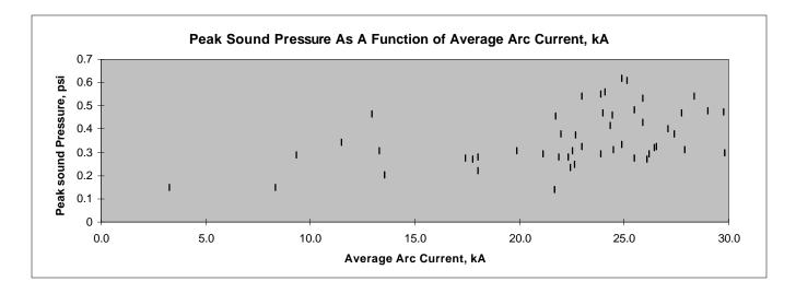
FIGURE 13. Peak Sound Pressure Variation With Average Arc Current
