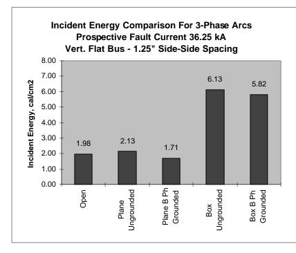
FIGURE 9. Incident Energy Comparison - 3-Phase Arcs With Vertical Electrodes In Flat Configuration
