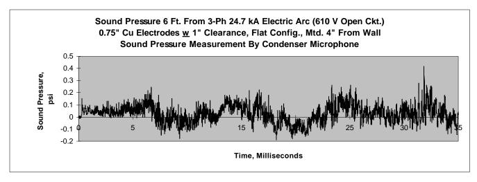
FIGURE 10. Typical Sound Pressure vs. Time Plot For A 3-Phase Electric Arc
