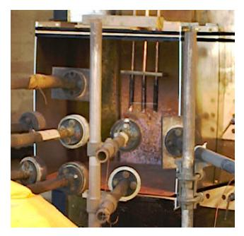
FIGURE 4. Test Setup No. 3 3 Phase Flat Electrodes In Box
