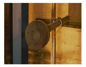
FIGURE 1. Copper Calorimeter On Test Stand
