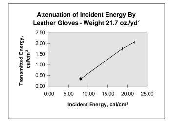
about 40% of the incident energy. Adding the polycarbonate faceshield further reduced the eye and **FIGURE 16. Leather Glove Protective Characteristics**
