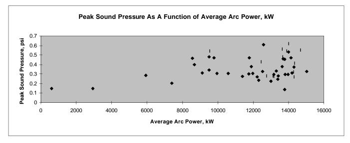
FIGURE 12. Peak Sound Pressure Variation With Average Arc Power
