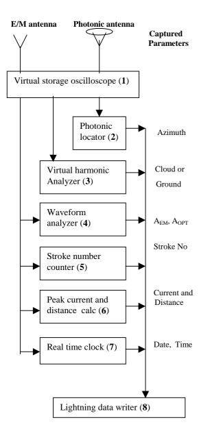
Fig.1.Lightning data acquisition block diagram.
