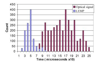
Fig.7. Optical signal half-width in comparison with LEMP zero-crossing time.
