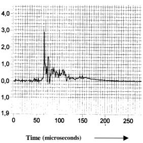
Fig.2. Typical "negative" ground return stroke waveform.
