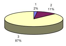
Fig. 6. Ground lightning polarity ratio. (1-"positive"; 2-"bipolar"; 3-"negative" strokes).
