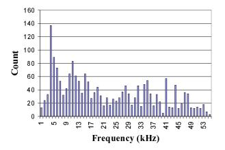
Fig.4. Ground lightning return stroke peak frequency distribution.
